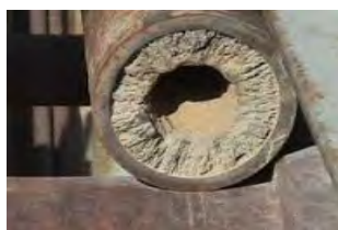
NORM scale in a pipe
