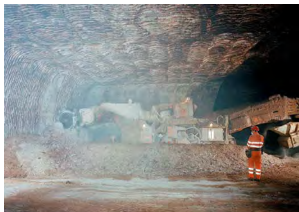
Plate 3-2 Example of continuous miner excavating rooms in a salt mine
