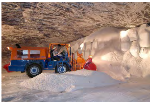
Plate 3-6 Salt backfill sprayer placing fine salt around waste packages
